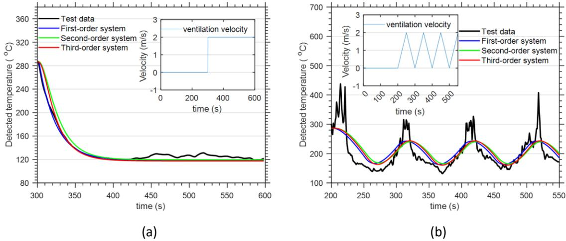
Figure 2 The plant model is obtained by system identification:(a) identification of the plant model; and (b) the validation of the plant model. The test data is the response curve with the input signal of ventilation velocity, which is calculated in FDS. Three systems of different orders (mathematically expressed) are used to approximate plant models.
