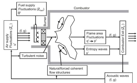
**Figure 1.** TRIGGERING MECHANISM OF THERMO ACOUSTIC INSTABILITY [1]
