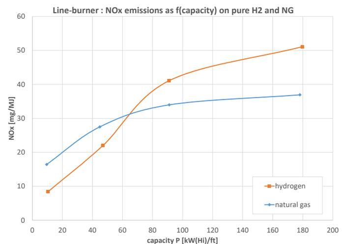
H2. Upgrading the burner with higher grade mix plates is the only modification required to fire the burner on hydrogen.
