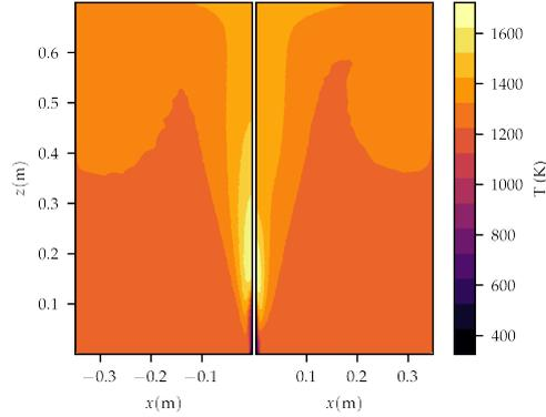
Figure 2: (*left*) Numerical distribution of the temperature for case 1. (*right*) Predicted temperature field using few experimental temperature samples.
