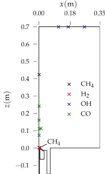
Figure 1: Optimal sensor placement inside the furnace.
