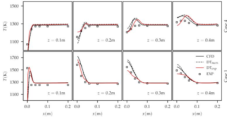
Figure 3: Temperature distribution for case 1 and case 4 at different positions along the axis. The averaged experimental uncertainty is 10 K.
